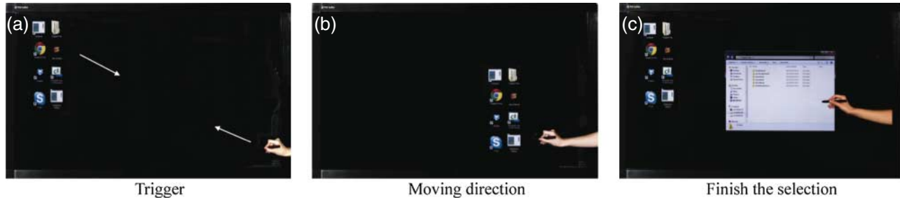
Figure 1. ShifTable: (a) the user draws an initial line with a finger or a pen to trigger the technique. (b) The user keeps moving the finger towards the desired target, and the screen shifts at a faster rate towards the finger. When it approaches, the target is selected by single tapping on it. (c) Then, the corresponding application is activated, and the screen returns automatically to its original position.
